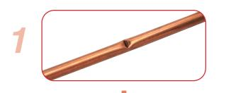
Ensure that the damaged pipe is kept clean
